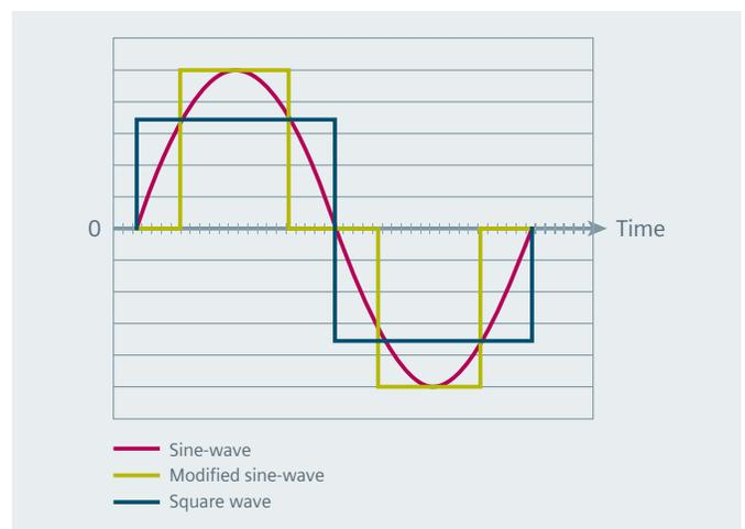
Figure 1: Two- and three-level output waveforms
