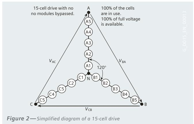
Figure 2 — Simplified diagram of a 15-cell drive
