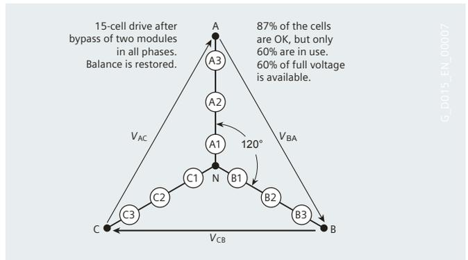
Figure 4 — Bypassing functional cells to rebalance drive output
