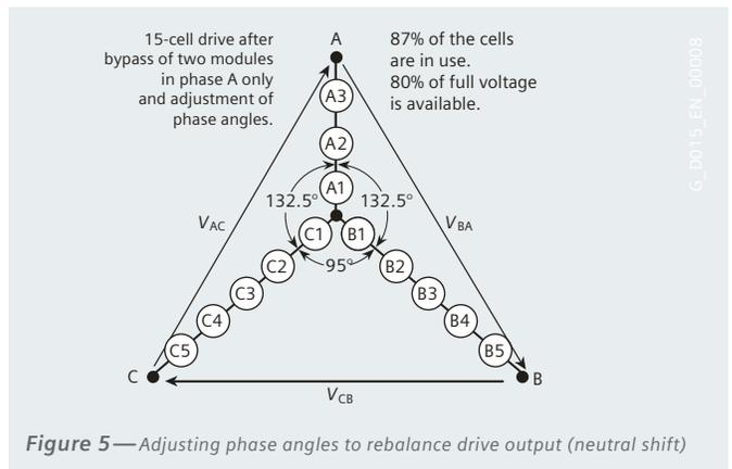
Figure 5 — Adjusting phase angles to rebalance drive output (neutral shift)
