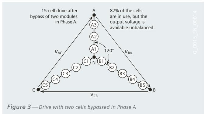
Figure 3 — Drive with two cells bypassed in Phase A
