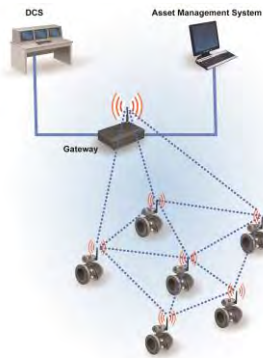
WirelessHART using mesh network technology.
