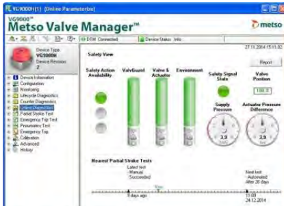
This DTM by Metso provides an easy to read graphical interface to help you migrate to a predictive maintenance
