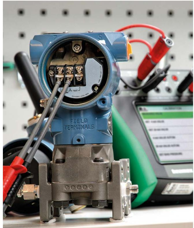
For a real metrological calibration, a traceable reference standard (calibrator) is always needed.
