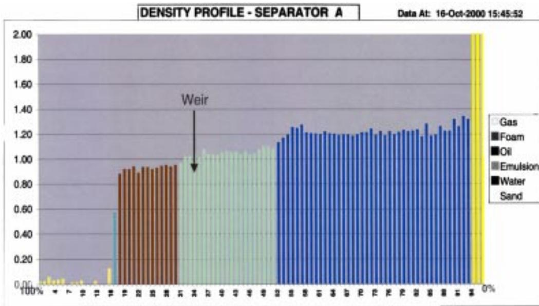
Figure 4: Actual screen dump of profile showing separator phase levels. 0% representing the bottom of the vessel and 100% the top.
