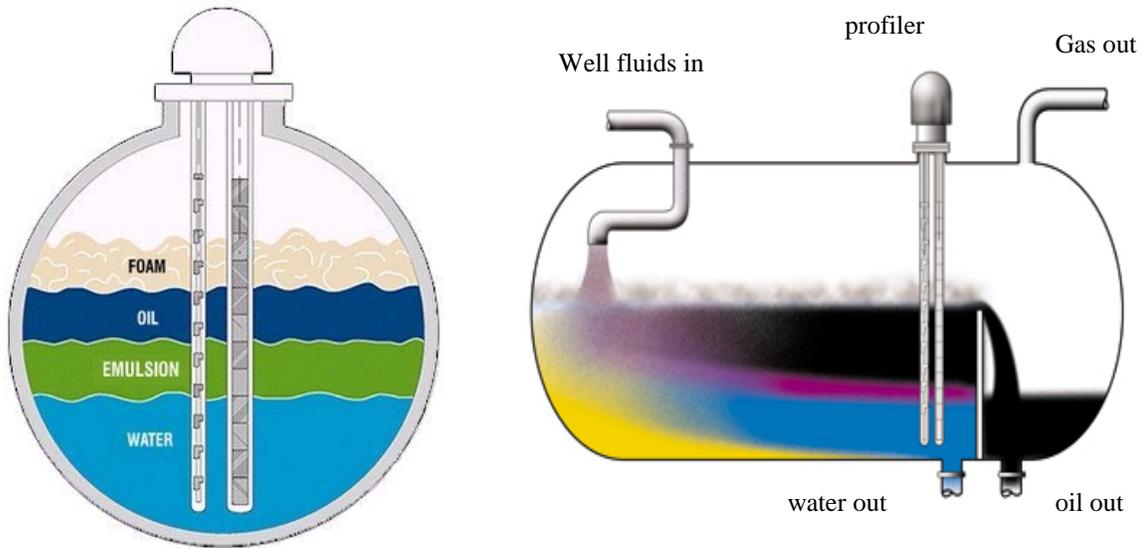
Figure 2: Views of profiler in vessel
