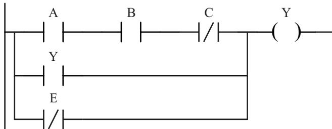
Figure 2.13. Output that appears as an input.
