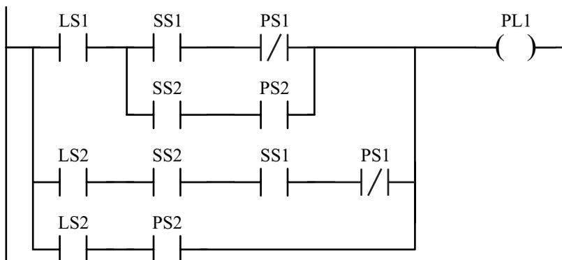
Figure 2.17. Reverse power flow in ladder logic corrected.
