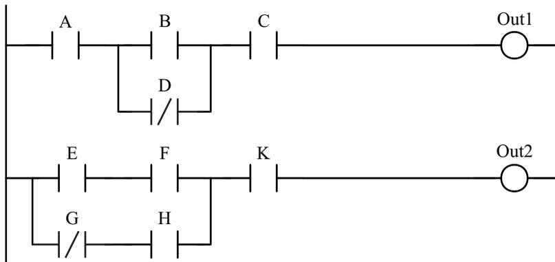
**Figure 2.7.** Ladder logic diagram with basic instructions.
