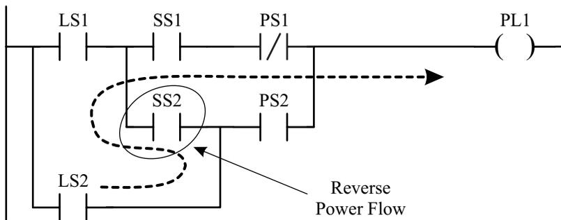
Figure 2.16. Reverse power flow in ladder logic.
