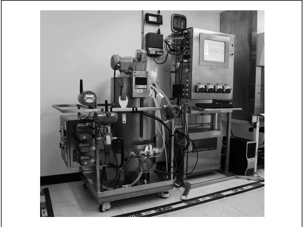
Figure 1-1. Portable Bioreactor with Wireless Industrial Instrumentation and a Lab Optimized DCS (Courtesy of Broadley-James Corporation)
