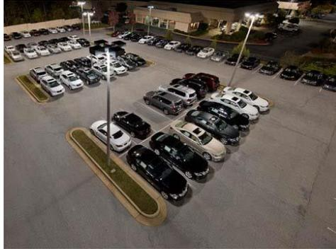
1000 Watt Metal Halide producing 22.9 measurable foot candles
