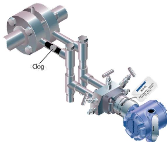
Figure 6: Diagram of Plugged Impulse Lines
