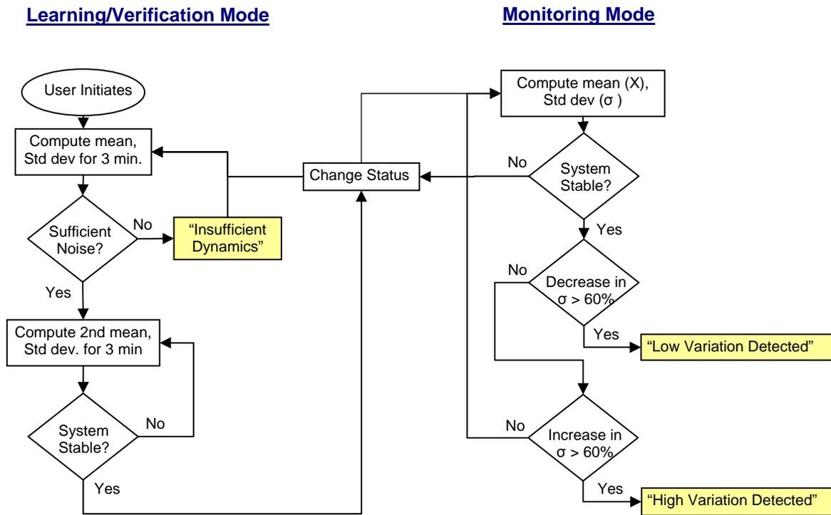
Figure 4: Simplified flowchart of SPM operation
