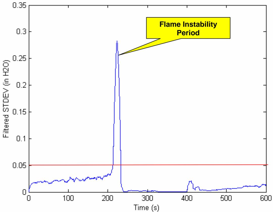
Figure 8: Standard deviation of Firebox draft pressure signal, after filtering in the 3051S HART Pressure Transmitter with Advanced Diagnostics.
