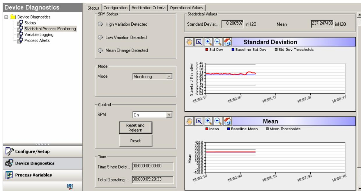
Figure 5: AMS Device Manager Enhanced EDDL SPM status screen.
