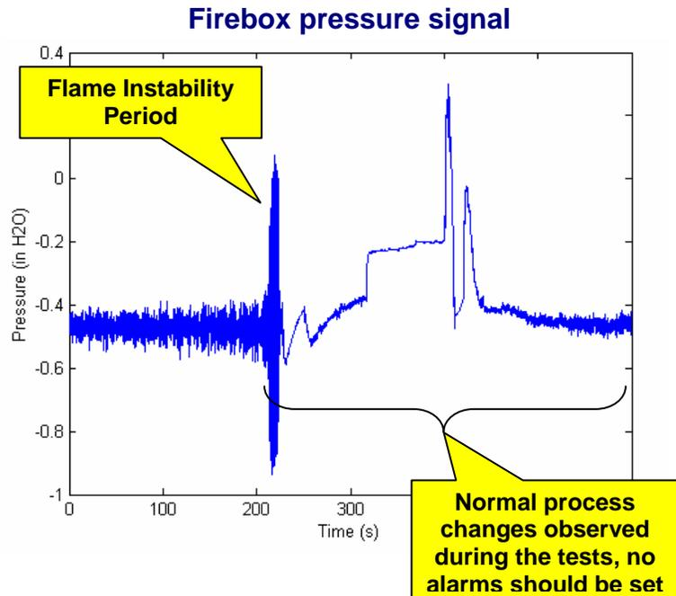
Figure 7: Refinery furnace and firebox pressure signal during tests, including period of flame instability
