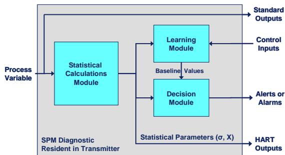
Figure 3: SPM block diagram
