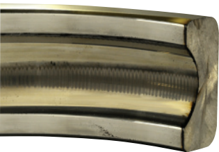
Fluting of a bearing race caused by bearing currents (Photo courtesy of Electro Static Technology).
