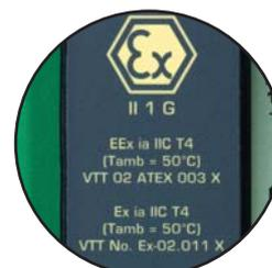
Marking on Beamex MC5-IS
