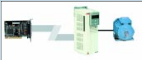
Figure A. The analog interface uses a separate wire for each signal between the controller and the drive. There may be up to 25 wires for each drive.
