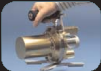
Livermore and Berkeley's 10-lb portable Cryo3 radiation detector.
